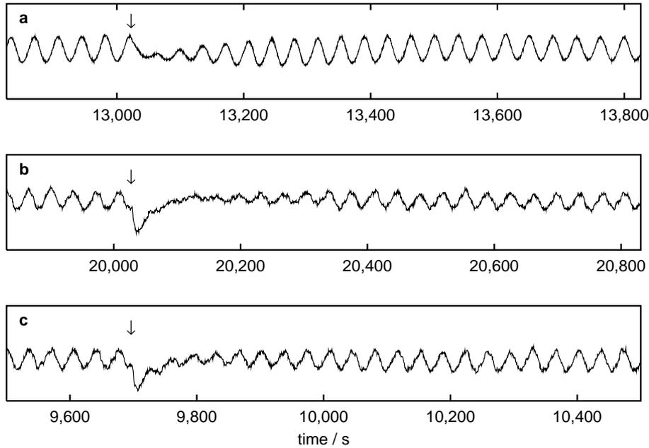
Fig(4) Quenching experiments (a) by addition of the optimal amount of glucose at the optimal phase and (b) by addition of the optimal amount of acetaldehyde at the optimal phase, and (c) addition of optimal amount of acetaldehyde 8° after the optimal phase.
