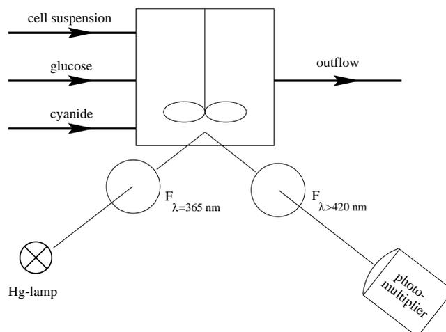
Fig(1). Experimental equipment. Dormant cells, glucose, and cyanide flow into the reactor. The concentration of NADH is monitored by observing the fluorescence of NADH from cells close to the cuvette surface.
